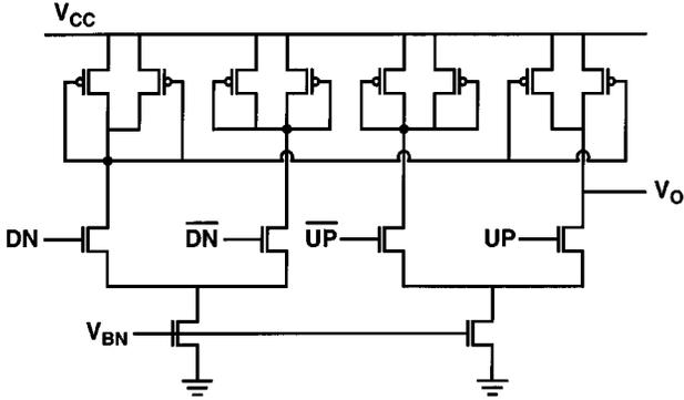
Fig. 8. Complete schematic of the offset-cancelled charge pump with symmetric loads.
