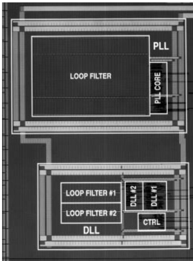
Fig. 16. Die micrograph of the dual-loop DLL and PLL.
