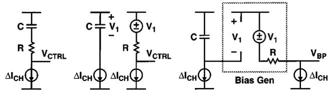
Fig. 11. Transformation of the loop filter for the integration of the loop filter resistor.
