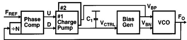
Fig. 12. Complete self-biased PLL block diagram (clock distribution omitted).
