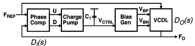
Fig. 3. Typical DLL block diagram (clock distribution omitted).
