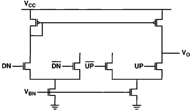
Fig. 7. Simplified schematic of the offset-cancelled charge pump.
