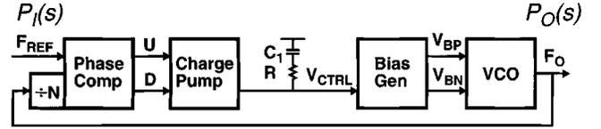
Fig. 9. Typical PLL block diagram (clock distribution omitted).
