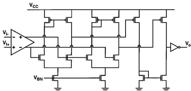
Fig. 15. Differential-to-single-ended converter with 50% duty cycle output.
