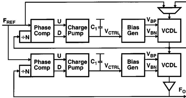
Fig. 17. Dual-loop DLL block diagram.
