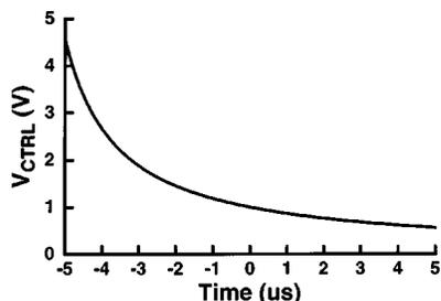
Fig. 13. Self-biased PLL control voltage as a function of time during capture.
