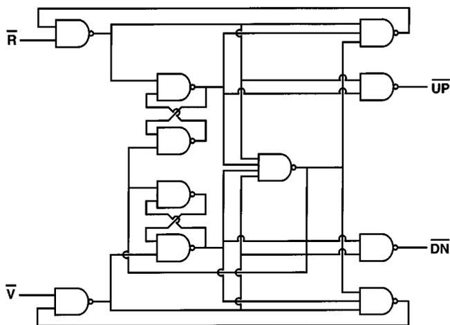
Fig. 14. Phase-frequency comparator with equal short duration output pulses for in-phase inputs.
