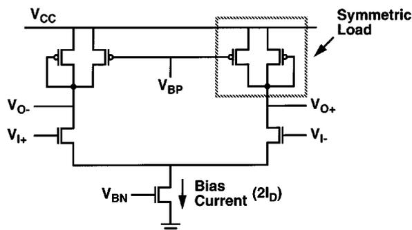
Fig. 1. Differential buffer delay stage with symmetric loads.
