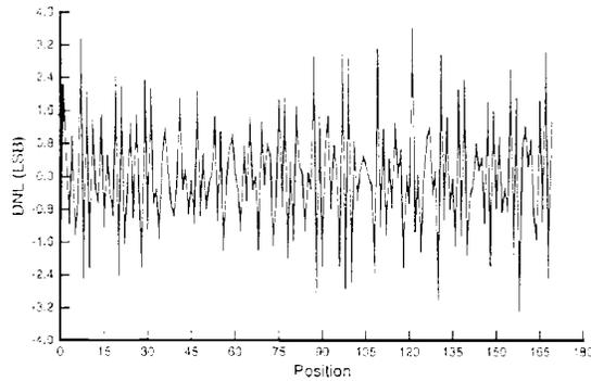
Figure 6: Differential non-linearity (23MHz, -22 mode).
