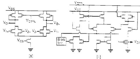
Figure 2: (a) Dual input differential buffer stage. (b) Current source bias circuit.
