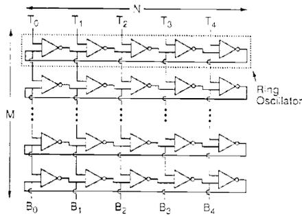
Figure 1: Array oscillator structure. All wires represent differential signal pairs.
