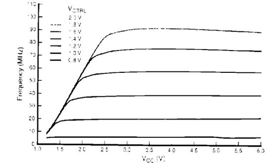
Figure 7: Frequency sensitivity to static supply voltage (-12 mode). At higher control voltages, changing die temperature causes a slight increase in frequency as the supply voltage is reduced.
