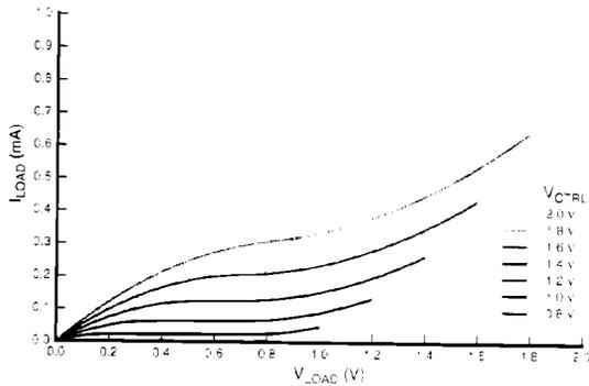
Figure 3: Simulated symmetric load I-V characteristics.
